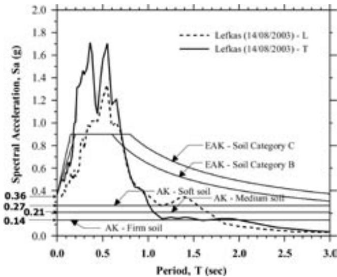
**Figure 6.** Elastic response spectra of the Lefkada main-shock ( $D=5\%$ ), recorded at the town of Lefkada, in comparison with the elastic design spectra of the old (AK) and recent (EAK-2000) Greek seismic codes, for different soil categories.
