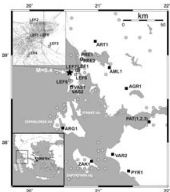
**Figure 4.** Permanent and temporary strong motion array of ITSAK deployed in the broader epicentral area (black squares: permanent network; gray squares: temporary array deployed after August 15, 2003). Lefkada mainshock is denoted by star. Earthquakes with  $M \geq 6$  are denoted with gray circles. The upper left inset shows the special array deployed within the town of Lefkada.
