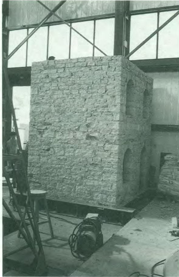
Figure 3. A building tested at LEE (stone masonry and arches)
