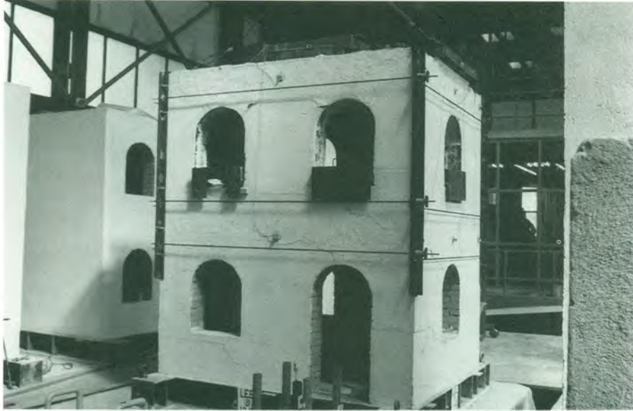
Figure 8. LEE building strengthened by vb-ht-a2, after a moderate shock
