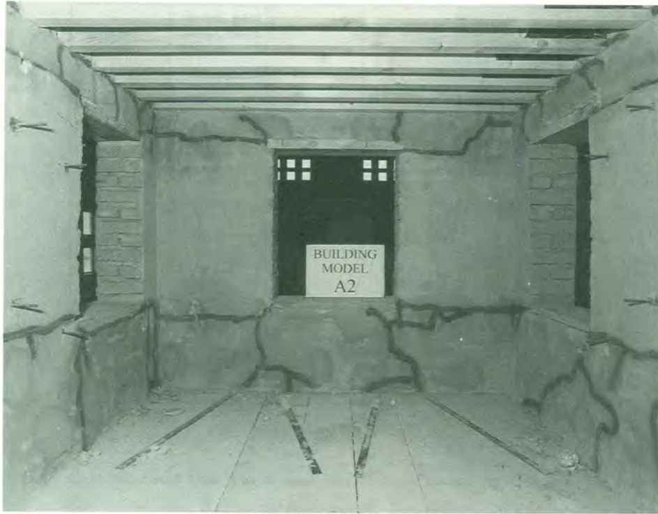
Figure 11. Heavy damage at the bases of piers at the first storey
